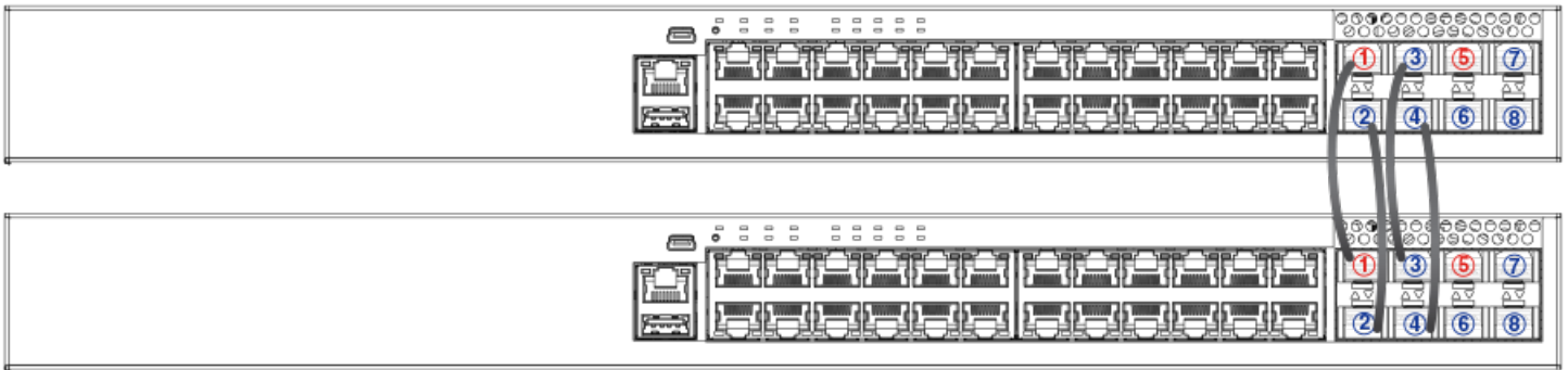
FIGURE 2 ICX 7250-24P Two-unit Stack with Linear-topology Trunk as Configured in Example
