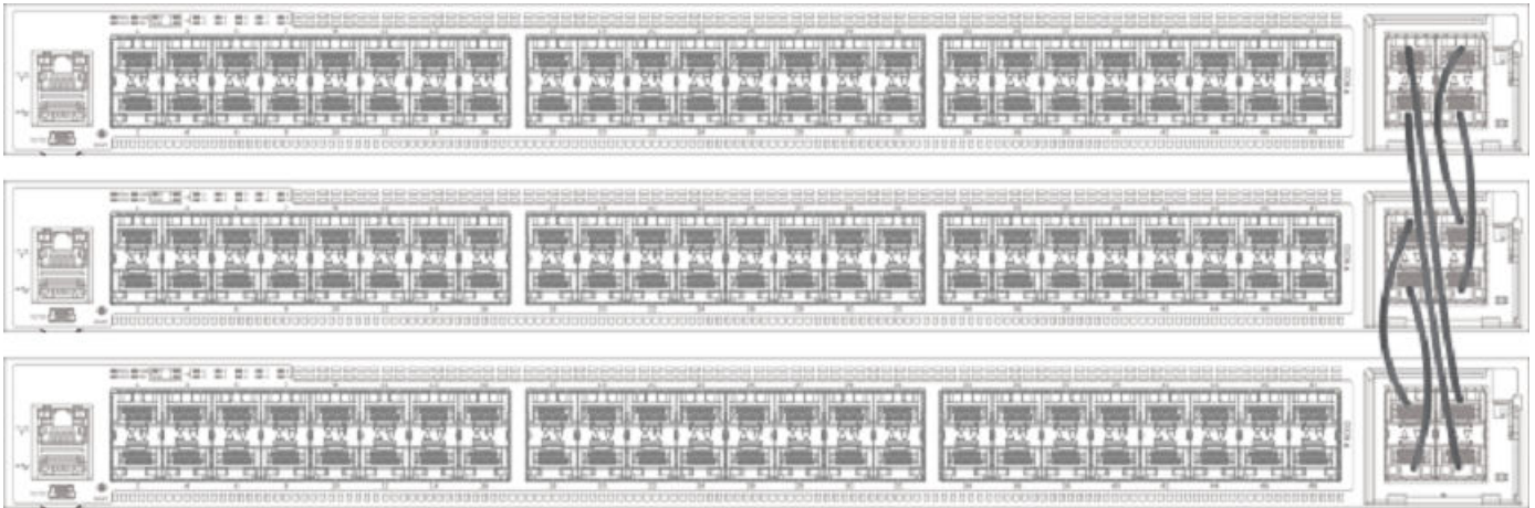
FIGURE 21 ICX 7450 4 X 10-Gbps Ring Using Stacking Trunks
